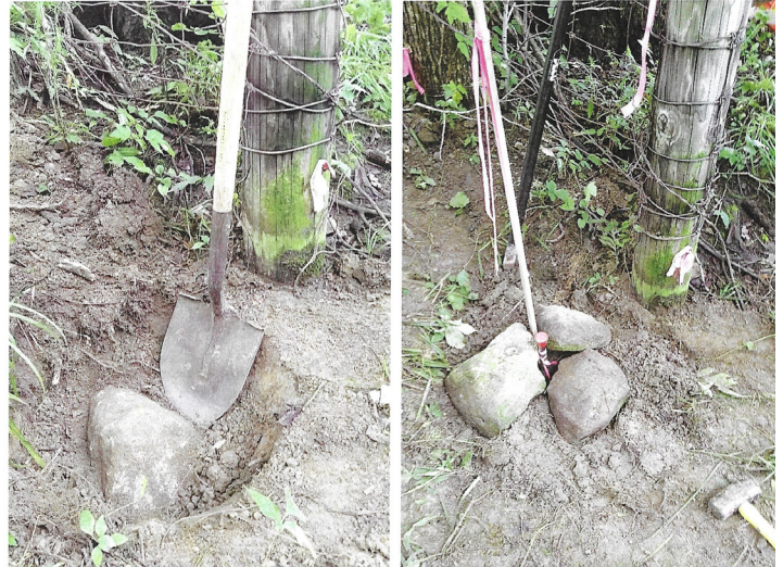
Above: Late 1800s monument stones used to delineate corners, found on Section 28/Section 29 boundary in Trowbridge Township in Allegan County in 2015.
