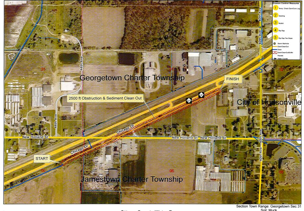
Ottawa County Water Resources Blacklock Ext.Drain Clean Out Section Town Range: Georgetown Sec Soil: Muck Length:2500 ft Cleanout Drain length:N/A Easement: 40ft
