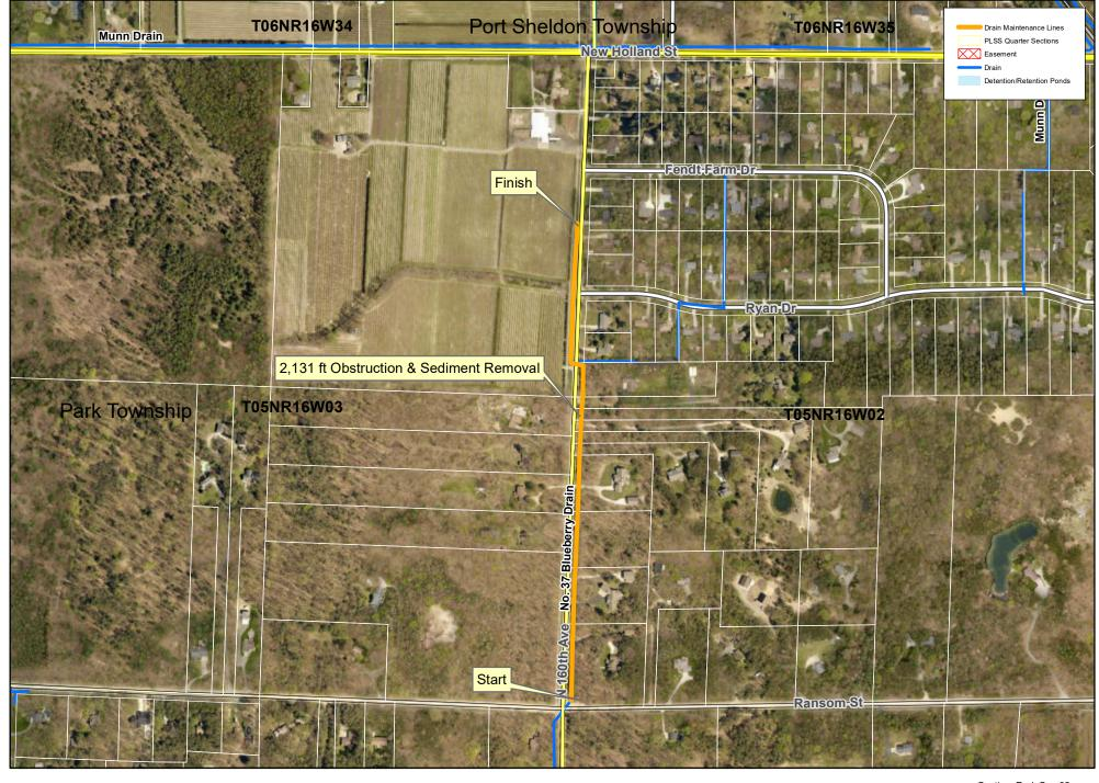
Ottawa County Water Resource No. 37 Blueberry Drain Clean Out Section: Park Sec 02 Soil: Length:2131 ft Cleanout Drain length:4870 ft Easement:0 ft
