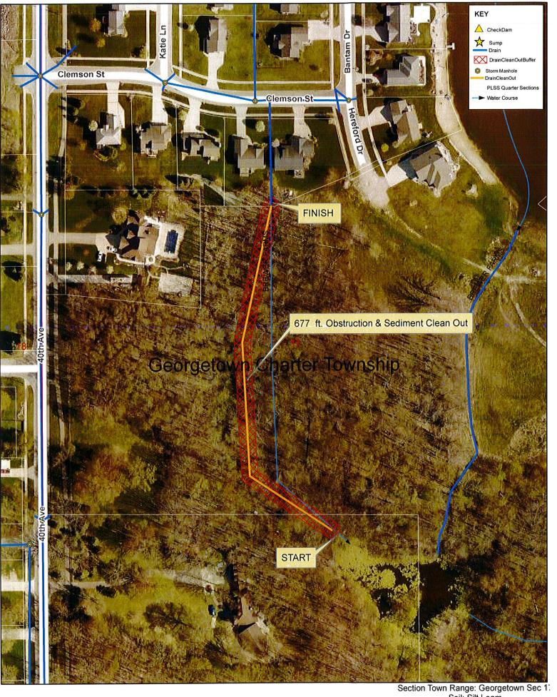
ction Town Range: Georgetown Sec 1 Soil: Silt Loam Length:677 ft Cleanout Drain length:6750ft Easement: 15ft each side
