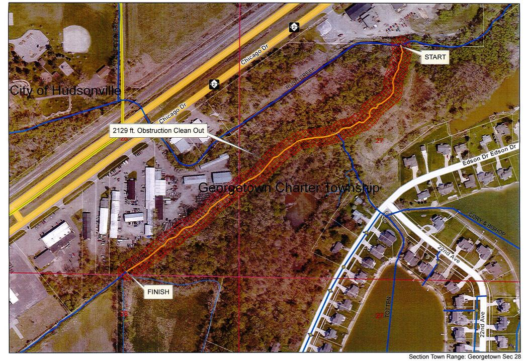
Ottawa County Water Resources Deweerd (Part 2) Drain Clean Out Section Town Range: Georgetown Sec 28 Soil: Loam fine sand Length: 2129 ft Cleanout Drain length:6,129 ft Easement:SG total
