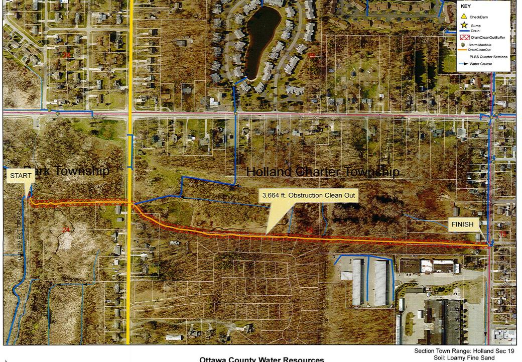
Ottawa County Water Resources No. 12 Drain Clean Out Section Town Range: Holland Sec 19 Soil: Loamy Fine Sand Length:3664 ft Cleanout Drain length: Easement: 50ft 25ft each side
