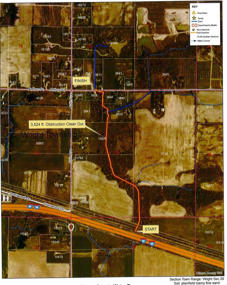
Ottawa County Water Resources Walz Drain Clean Out Section Town Range: Wright Sec 29 Soil: plainfield loamy fine sand Length: 3,524 ft Cleanout Drain length: 4,701ft Easement: 16ft each side
